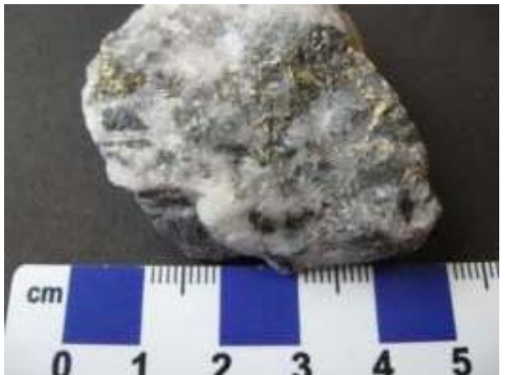
Figure 1 This sample from Engineer Mine shows gold in quartz found as float. It was retrieved from the lakeshore near the old mill. To view more samples go to the David K. Joyce Minerals website* at www.davidkjoyceminerals.com/pagefiles/engineermine.asp .
